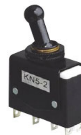
KN5-1 ON-ON SPDT 4P KN5-2 ON-ON DPDT 8P KN5-4 ON -OFF 4PST 8P 10A 125VAC 5A 250VAC
